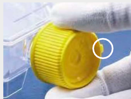
VENT position at 3 o'clock = gas tight
